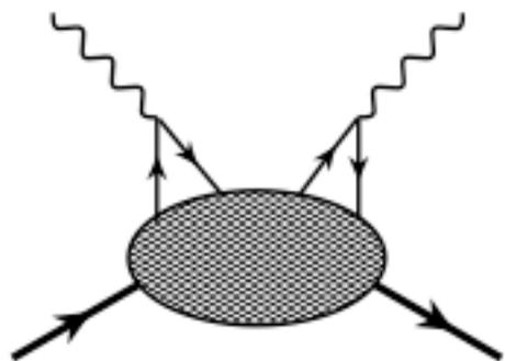
cat's ears diagram (4-fermion higher twist  $\sim 1/Q^2$ )
