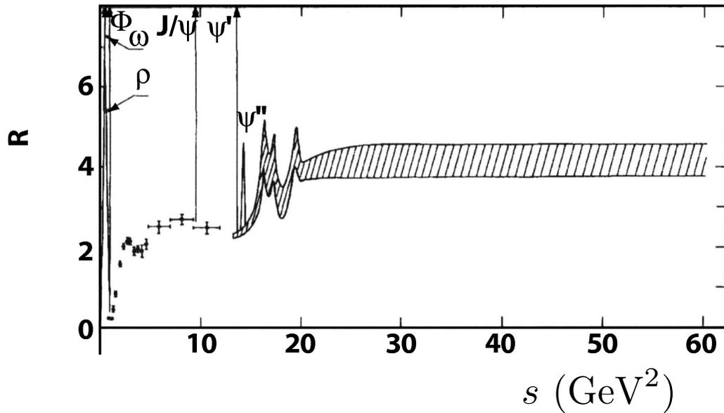
$$R = \frac{\sigma(e^+e^- \rightarrow \text{hadrons})}{\sigma(e^+e^- \rightarrow \mu^+\mu^-)}$$
