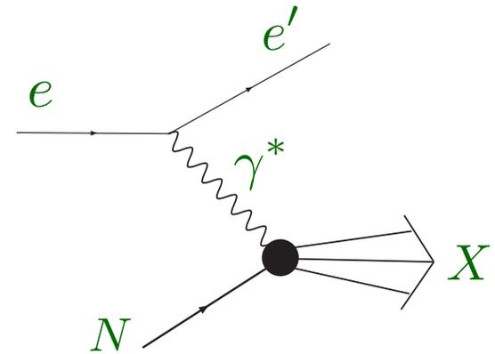
$$\left. \begin{aligned} \nu &= E - E' \\ Q^2 &= \vec{q}^2 - \nu^2 = 4EE' \sin^2 \frac{\theta}{2} \end{aligned} \right\} x = \frac{Q^2}{2M\nu}$$
